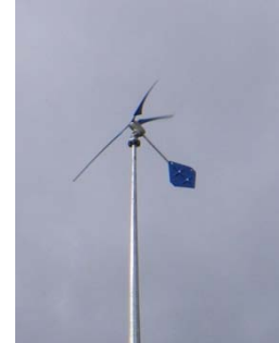
The wind turbine tilts to protect itself in high winds, but is still producing power
